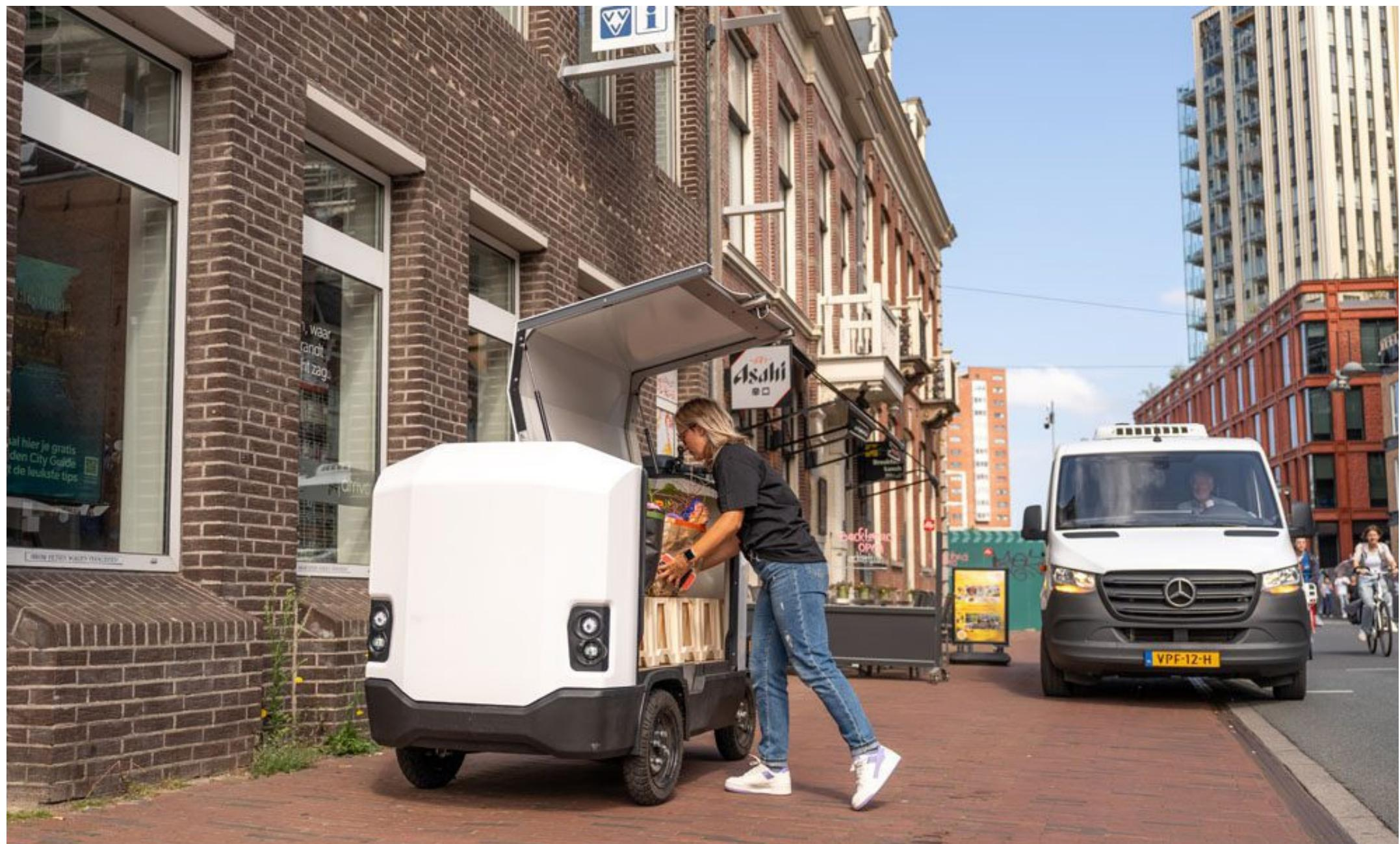
> The cargo space can fit 250 kg of cargo and has a volume of 1.2 m<sup>3</sup>. A compartment under the floor offers space for a spare tire and additional storage.
