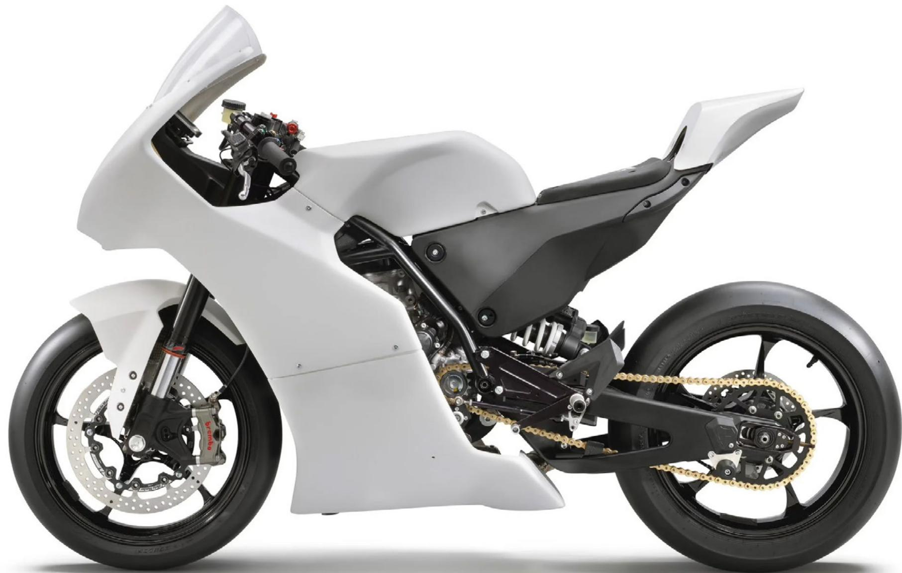
> The chassis design has the ability to be adjusted at the headstock angle, triple-clamp offset, swingarm angle, seat height, rearset height, and handlebar angle.
