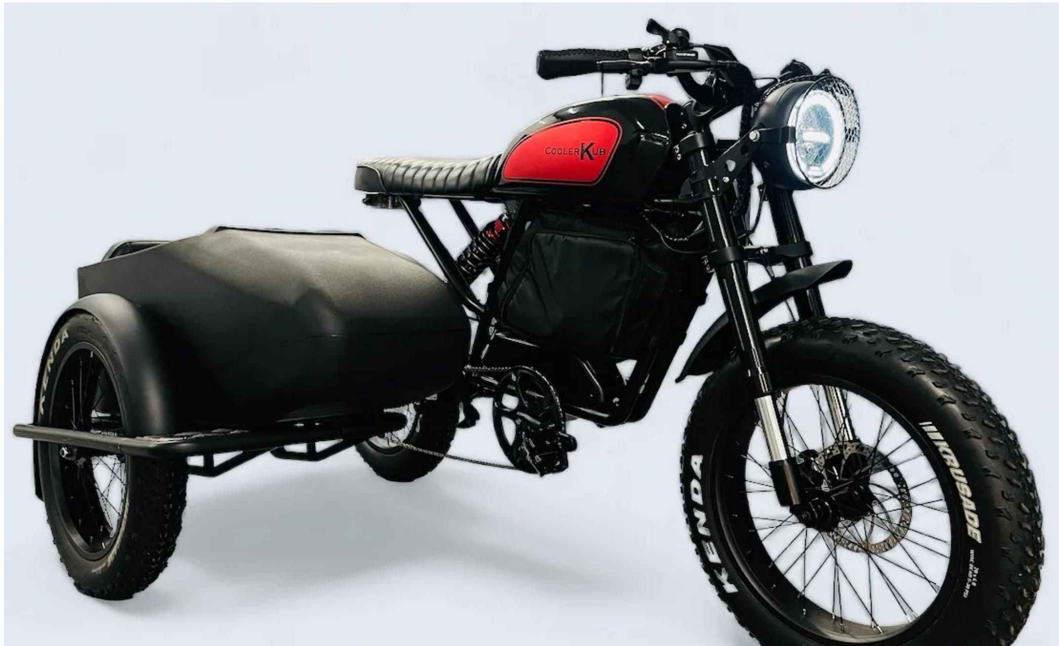
> The sidecar is rotomoulded in a single piece and mounted on the metal frame.
