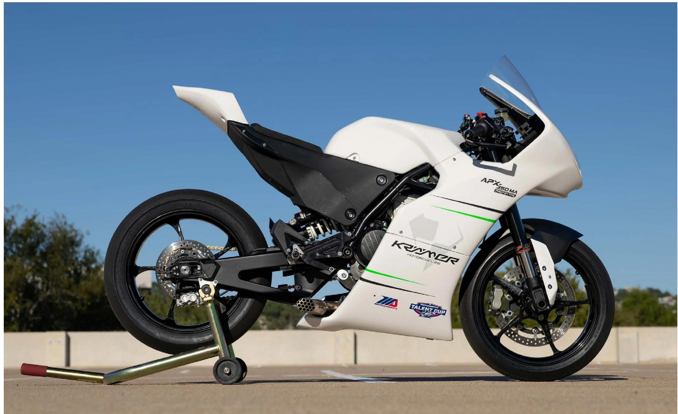
> The Krämer APX-350 MA features a 350cc single-cylinder engine from the KTM EXC-F enduro motorcycle.
